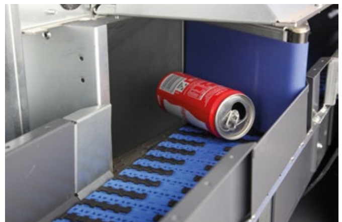
The switch redirects the empty container
